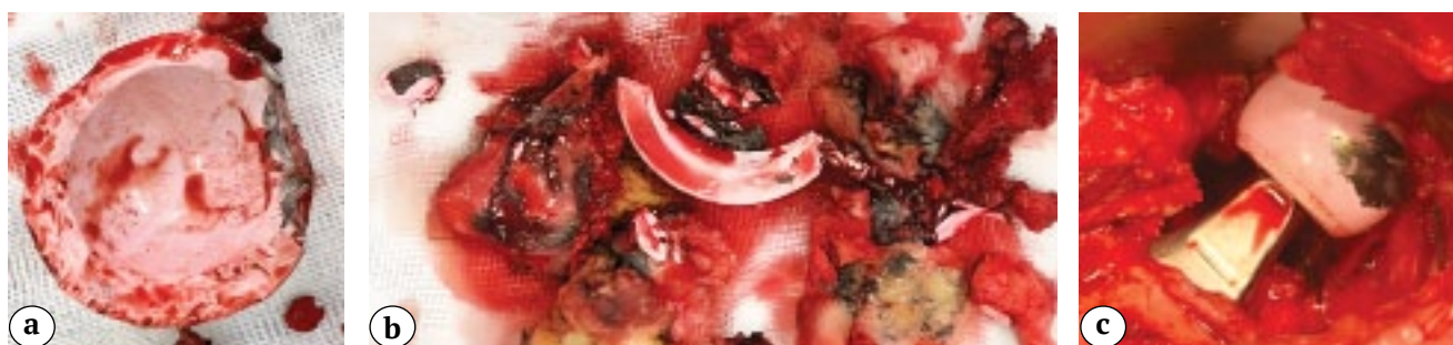
Fig. 5. The appearance of the ceramic liner fragments: a — a large ceramic liner fragment (central) 20×20 mm with signs of metal contact (black); b — medium (15×6 mm) and small fragments (2×3 mm) with excised surrounding tissues; c — femoral head with signs of metal contact (black)
