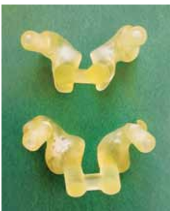
Fig. 2. Navigation templates for pedicle screws placement in vertebrae plastic models
