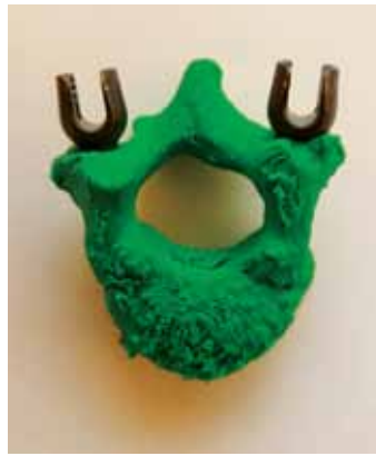
Fig. 3. Vertebra plastic model with pedicle screws placed with the use of navigation templates
