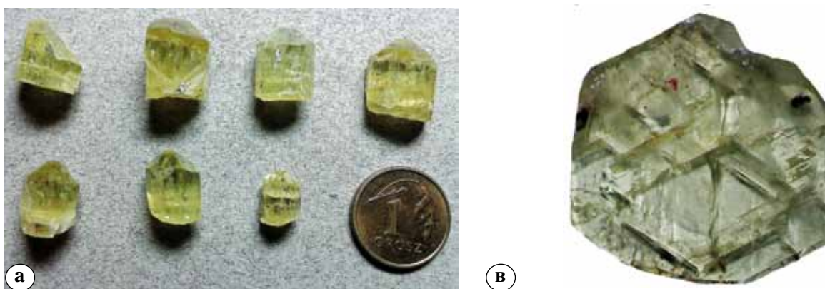
Fig. 1. Crystals of apatite from Morocco used in the first experiment (A); picture of a plate of apatite cut perpendicularly to optical axis Z (B). Visible are inclusions and a net of cracks (enlarged \times 10 )
