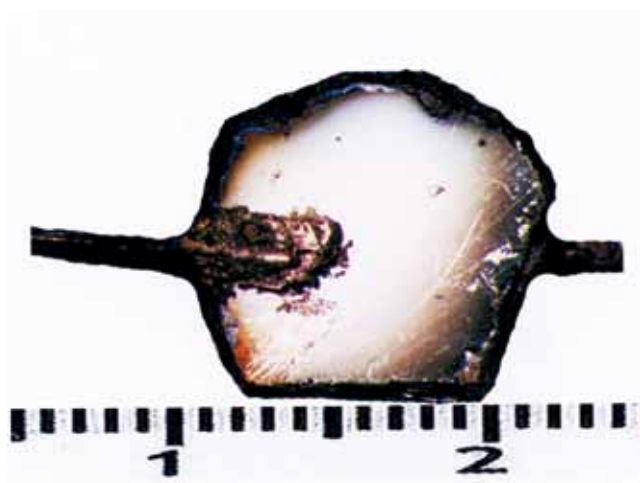
Fig. 4. Example image of an apatite plate cut perpendicularly to the optical axis Z after dusting with gold. The dark edge is a paraffin border; after dusting with gold and removal of the border, upper and lower surfaces of the plates were electrically separated.
