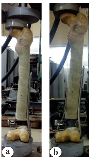
Fig. 1. Simulated fracture models with mounted motion sensors: а – first series with lateral fixation; б – second series with bilateral (lateral and medial) fixation
