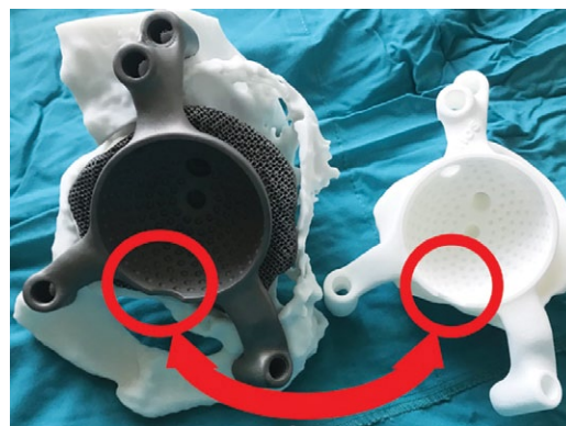
Fig. 3. Custom-made pelvis fragment, component, and trial model of the acetabulum. The red circle indicates an additional recess at "6 o'clock" for optional orientation during implant positioning
