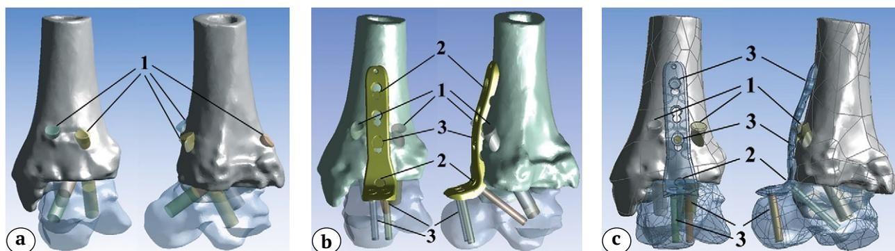
**Fig. 2.** 3D models in two projections (frontal and lateral) of ankle arthrodesis: a – with three cancellous screws; b – the originally designed plate and two cancellous screws, the proximal screw is cortical; c – the originally designed plate and two cancellous screws, proximal screw with angular stability 1 – cancellous screw, 2 – cortical screw, 3 – screw with angular stability
