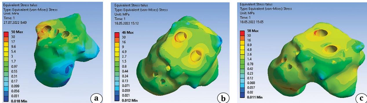
**Fig. 8.** Equivalent stresses in the talus during loading simulating dorsiflexion of the foot, MPa:
