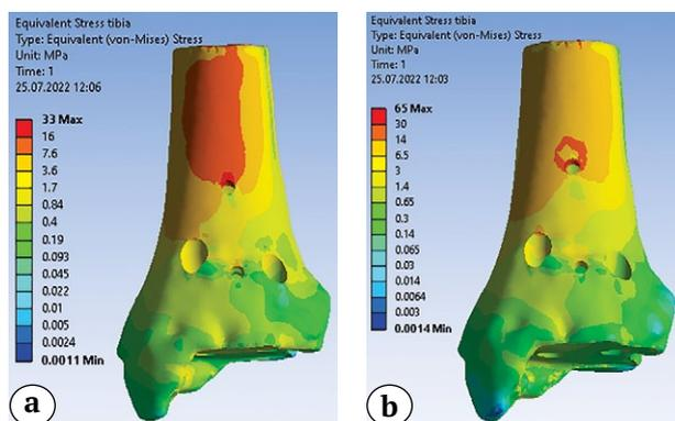
**Fig. 9.** Equivalent stresses in the tibia during a load simulating dorsiflexion of the foot, MPa:
