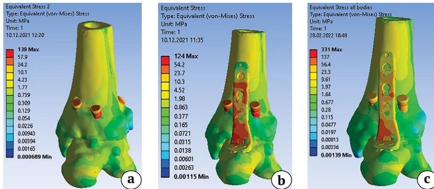
**Fig. 7.** Equivalent stress fields for dorsiflexion models, MPa:
