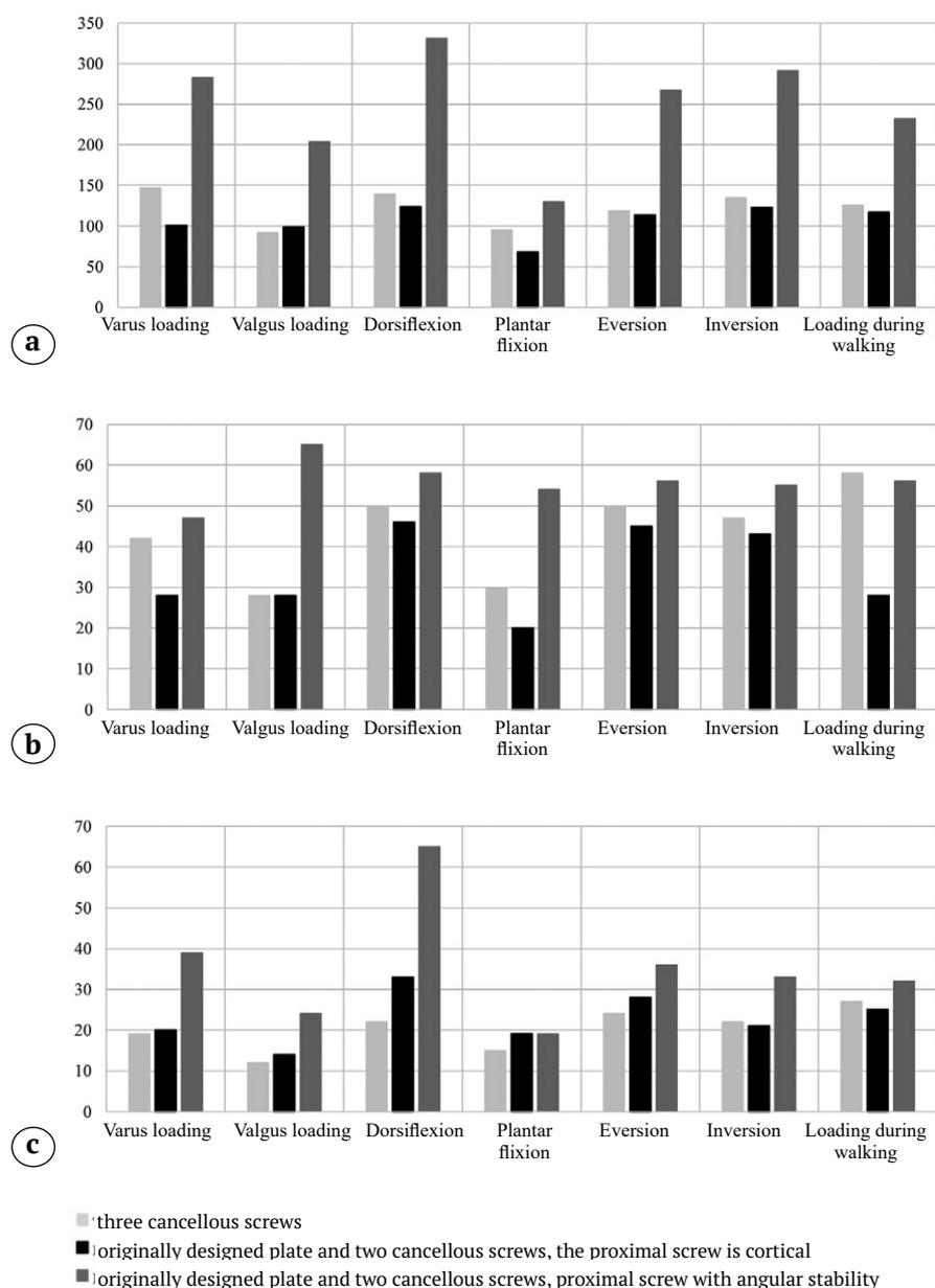
**Fig. 4.** Maximum equivalent stresses for various types loads of on the ankle joint, MPa: a – in the studied implants; b – in the talus; c – in the tibia
