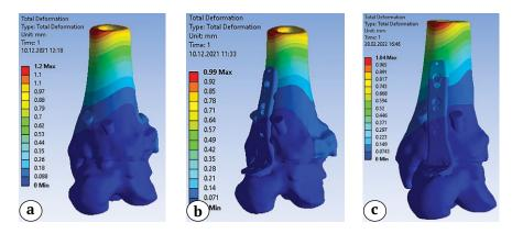
Fig. 6. Total displacement fields for three models of dorsiflexion fixation, mm:
