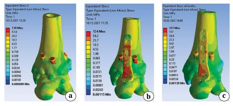
Fig. 7. Equivalent stress fields for dorsiflexion models, MPa:
