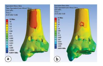
**Fig. 9.** Equivalent stresses in the tibia during a load simulating dorsiflexion of the foot, MPa: a – second option; b – third option
