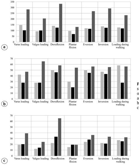
**Fig. 4.** Maximum equivalent stresses for various types loads of on the ankle joint, MPa: a — in the studied implants; b — in the talus; c — in the tibia
