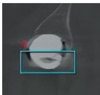
Fig. 4. MSCT, sagittal projection: fracture of the ceramic liner
