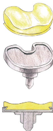
Fig. 6. Peripheral type of fixation of the polyethylene insert in the tibial component of the knee endoprosthesis
