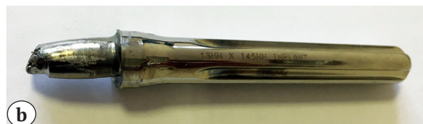
Fig. 2. The removed metaepiphyseal part of the femur and the femoral component of the endoprosthesis (a); broken intramedullary stem of the femoral component (b).
