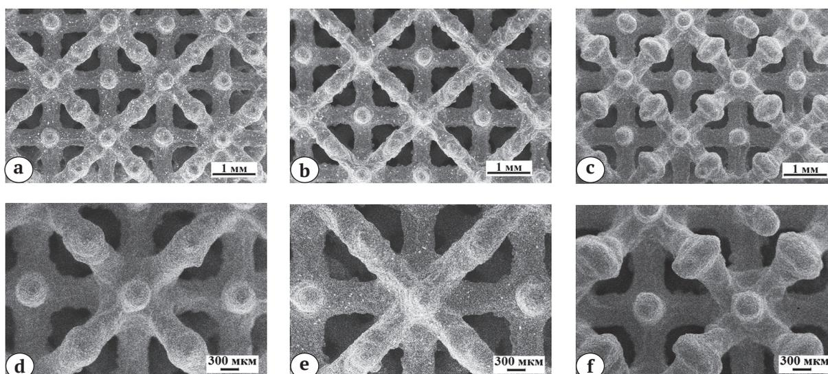
**Fig. 2.** SEM images of the porous implants structures made by DMLS: types I (a, d); types II (b, e); types III (c, f). Magnification:  $\times 50$  (a, b, c),  $\times 100$  (d, e, f).
