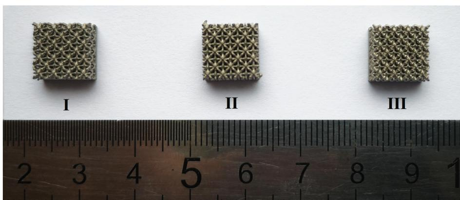
**Fig 1.** Samples of the porous materials made by DMLS.
