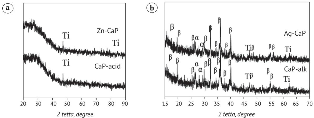
**Fig. 6.** X-ray coatings placed in the acidic (a) or alkaline electrolytes (b): Ti – titanium;  $\alpha$  –  $\alpha$ -TCP;  $\beta$  –  $\beta$ -TCP, TCP = tricalcium phosphate.
