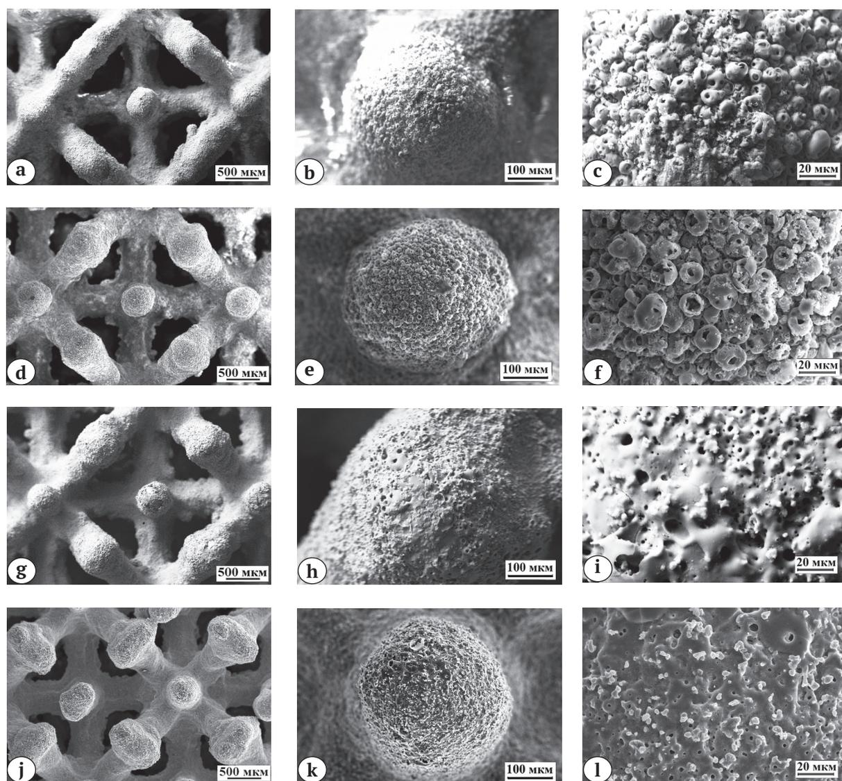
**Fig. 3.** SEM images of the porous implants coatings: CaP-acid (a, b, c), Zn-CaP (d, e, f), CaP-alk (g, h, i) and Ag-CaP (j, k, l). Magnification  $\times 100$  (a, d, g, j),  $\times 500$  (b, e, h, k),  $\times 2000$  (c, f, i, l).
