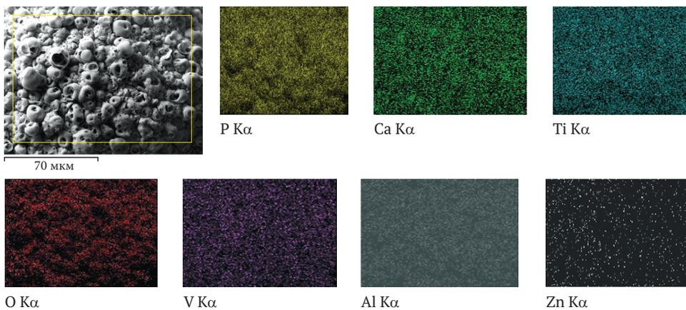
Fig. 4. SEM images and the elements distribution maps in the acidic calcium phosphate coating with Zn.
