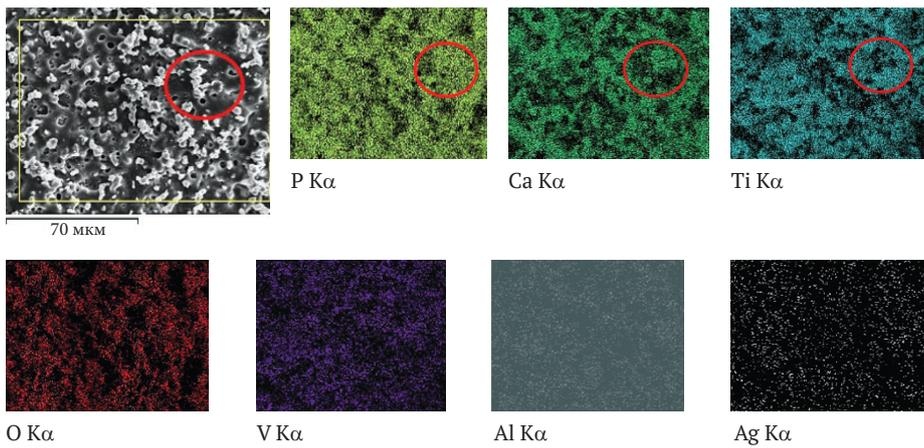
**Fig 5.** SEM images and the elements distribution maps in the alkaline calcium phosphate coating with Ag.
