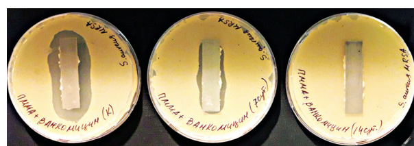
Fig. 3. Antibacterial activity of bone cement based coating impregnated with 5% vancomycin against the antibiotic-resistant clinical isolate of S. aureus 43431 (MRSA), a bilayer agar method
