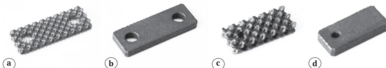
**Fig. 1.** Samples of titanium implants:
